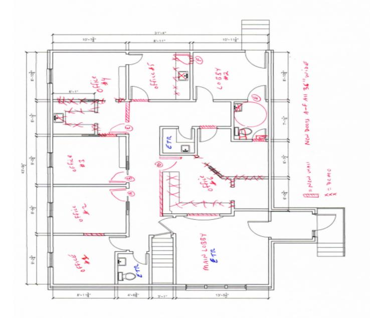
EXISTING FLOOR PLAN 1 SCALE: \$4"=1'-0" - ALL NEW LED LIJUTS (Sep permit) - NEW LED EMERCENCY LIGHT to Scinstilled UNDER Electrici PLAMIT AND VENES Smoke/enter Defectors 3/16 = 1 0 - DOUN AND WALL CHANGE IN RED MUVE TULL AND UNDER to improve wheel chain PATCH, PACP AND PAINT T use in Turktanin Charge All PYTONION Light build to LES - Repris Drop ceiling CONSTRUCTION SCOPE : - Replace All Flooring 2+ 49917 ı ι ı
